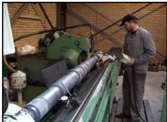
Grinding of larger shafts is outsourced, and we have refurbished shafts up to 5,600 mm in length.
